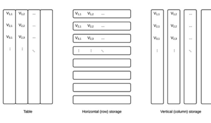
**Fig. 2.** Row vs. column oriented storage model.
