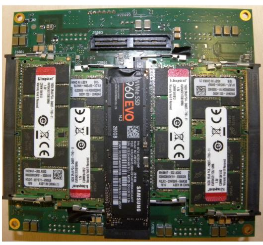
• 120x130 mm<sup>2</sup> board, 12 PCB layers, 1700 components, 46 power supplies, 16 power sensors
